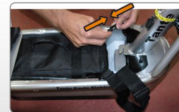
Take the battery out of the small carton and, if necessary, remove the transport retaining band from the plug. Use the ignition key to open the battery compartment and insert the battery. Then connect the two plugs, which for reasons of safety will require a bit of effort to connect.
