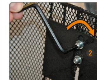
Remove the basket from the small carton and screw it to the mount on the seat tube.
