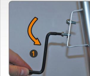
Remove the basket from the small carton and screw it to the mount on the seat tube.
