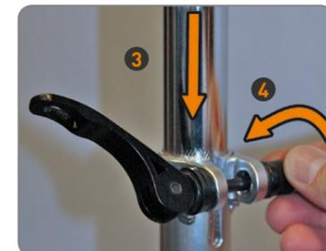
3 Push the seat with the seat post into the seat tube, leaving about 10 cm standing out.
