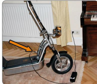
Connect the charger to a power point and to the charger port located below the ignition lock.
