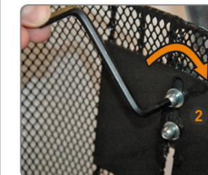
2 Place the basket on the mount, push the screws through the slot and fasten them to the mount. For safety reasons, the basket is elastic. Should it be deformed, push it back into shape with your hands.
