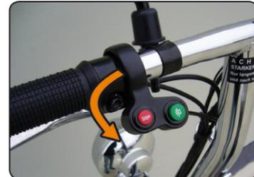
To adjust the angle, loosen the black screw on the brake lever with the included tool. You can then adjust the brakes as you wish. Make sure to tighten the screw again afterwards.
