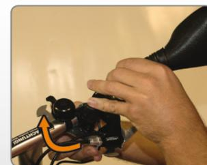
Remove the screw nut and the washer from the rear-view mirror. Open the clamp. Then, using the clamp, affix the mirror to the part of the handlebar protected by a fibre band. Arrange the mirror in an upright position and fasten it with the screw. Hold the mirror with one hand and fasten the screw nut with the included tool.
