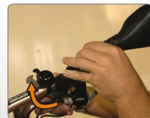
Remove the screw nut and the washer from the rear-view mirror. Open the clamp. Then, using the clamp, affix the mirror to the part of the handlebar protected by a fibre band. Arrange the mirror in an upright position and fasten it with the screw. Hold the mirror with one hand and fasten the screw nut with the included tool.
