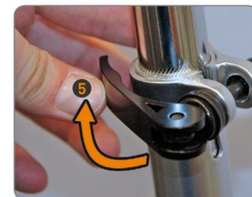
5 Fix the post by folding over the safety clasp. By opening the clasp, you may later change the seat height.
