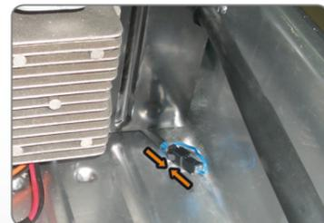
You'll find a small, black plug connector with a blue cable at the front of the battery compartment. If it is open, the scooter will accelerate gently. If you close this connection, the acceleration speed of the scooter increases.
