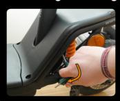
The scooter is delivered with one short and one long seat post. As delivered the seat is affixed to the long post. Select the seat post appropriate for your seat height and if required attach the seat and the reflector to the short seat post. Insert the desired seat post into the designated brackets on the scooter. Then screw it in tightly from the side.
