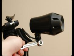
1) Align the front light in the direction of travel and 2 screw it in tightly on the side using the wrench and the T Allen wrench. Make sure not to bend the light bracket!
