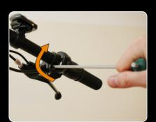
To adjust the angle, loosen the black screw on the brake lever with the included tool. You can then adjust the brakes as you wish. Make sure to carefully tighten the screw again afterwards.
