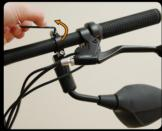
Remove the mirror from the small carton. Open the clamp with the included tool and then facing down on the left side affix the mirror to the part of the handlebar protected by a fiber band.
