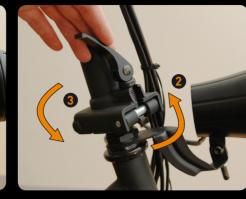
1 Before folding upright push the bolt to the side and then fold the handle-bar completely upright. Push the bolt back, 2 fold the securing screw with the spring upright and 3 then fasten the hinge with the black safety clasp.
